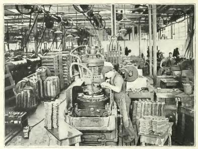
Photo from Colt's Patent Firearms Manufacturing Company MACHINING ROUGH PISTOL CASTINGS time. What was needed was a hand weapon that would put the adversary out of fighting the instant he was hit, whether fatally or not. We therefore increased the caliber of the automatic pistol to .45 and slowed down the bullet so that it tore flesh instead of making a clean perforation. These improvements gave the missile the impact of a sledge hammer, and a man hit went down every time.
