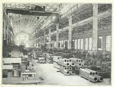
Photo from Otis Elevator Company MAKING 240-MILLIMETER RECUPERATORS
