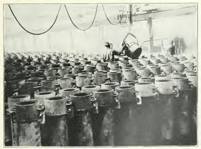
Photo from Willys-Overland, Inc. CASTING SHELL IN FLASKS
